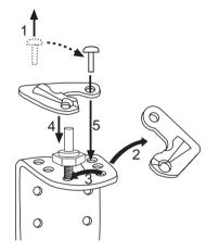
Remove the door fitting on the lower right (1) and reposition the door bearing cover from the lower left to the right of the door (2), place the door fitting supplied in the lower left of the door (3). Carefully remove the door to the front and place on one side.
